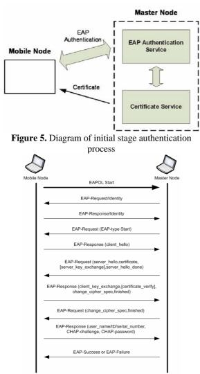
Figure 6. Initial stage EAP messages exchange
