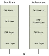
Figure 4. EAP multiplexing model
