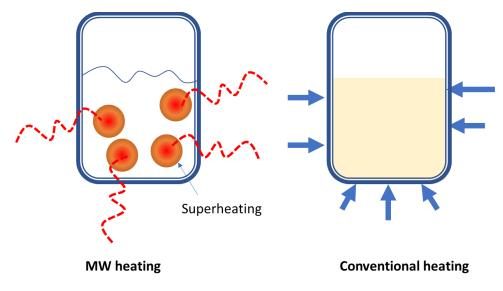
Figure 2. Differences in heat flow patterns in regular heating and MW
