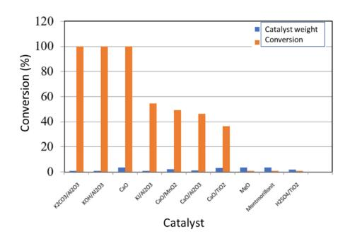
**Figure 5.** Effect of catalyst types on the methyl ester yield of sunflower seed oil (Reaction conditions of methanol: oil ratio = 16:1; Catalyst 10 wt.%; reaction time 2 hours, temperature 70 °C)
