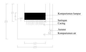
Gambar 2. Reaktor cacing
