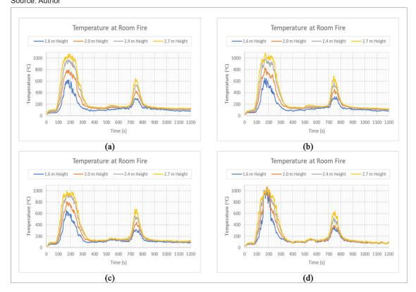
Chart 2. Room of fire temperature development in condition (a) no wind), with wind 0.5 m/s, (c) with wind 2 m/s, and (d) wind 5 m/s Source: Author
