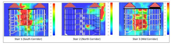
Figure 13. Wind velocity distribution at t = 180 s (Occupied level) Source: Author
