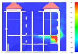
Figure 10. Temperature distribution at the room of fire (occupied level)
