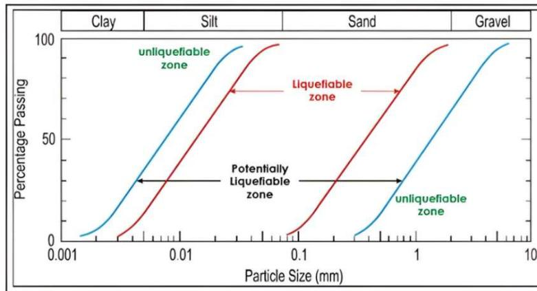
Figure 2. Curve of soil particle size distribution for susceptibility to liquefaction (Suprijanto et al., 2020)
