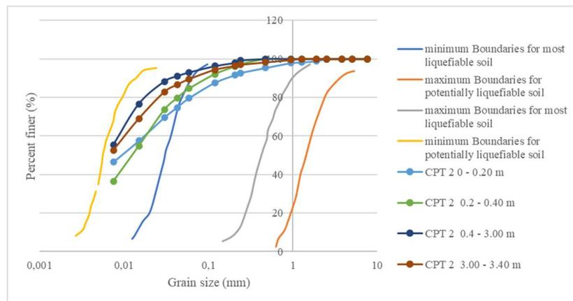
Figure 5. Liquefaction analysis in CPT 2 based on grain size analysis
