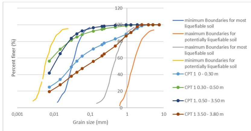
Figure 4. Liquefaction analysis in CPT 1 based on grain size analysis
