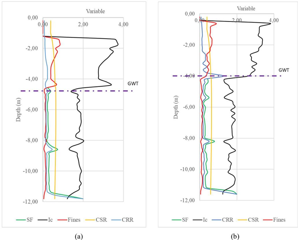
Figure 6(a). Liquefaction analysis based on CPT 1 Figure 6(b). Liquefaction analysis based on CPT 2
