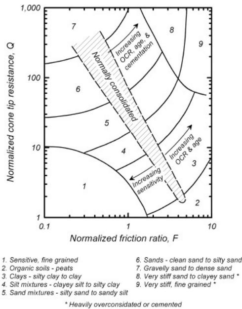
Figure 3. Correlation between Fr and Q (Idriss and Boulanger, 2008)
